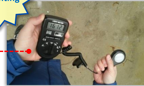
Underdeck Measurement After Deck Installation: 1,612 lux (Fluorescent Light 20W approximately 150 lux)
